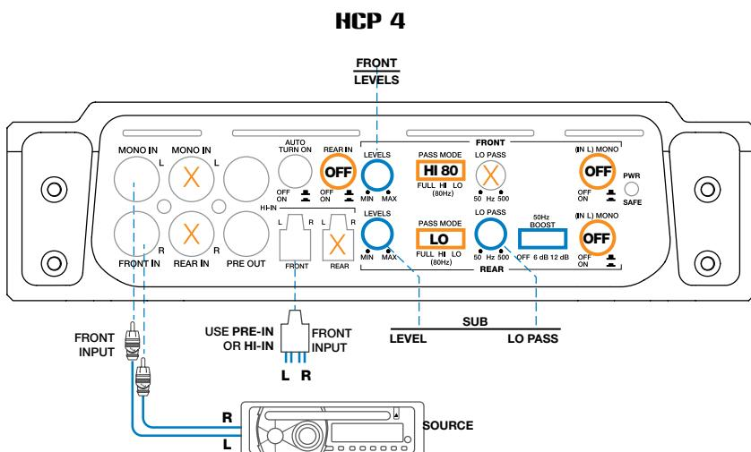
Using also REAR INPUTS to drive SUBWOOFER:
