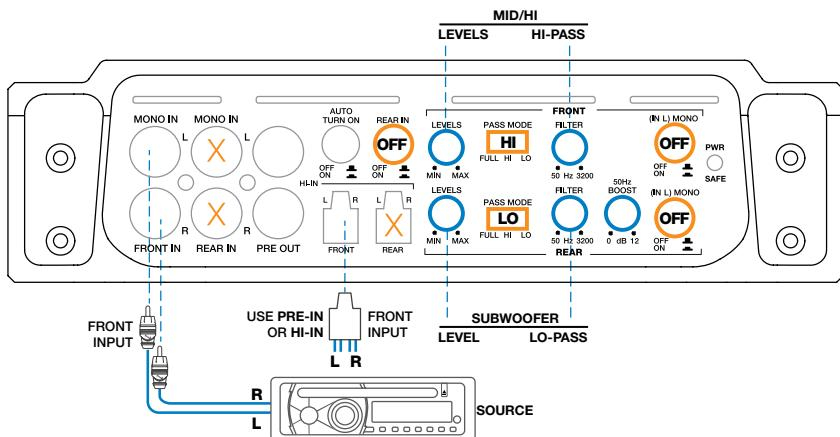
**Using also REAR INPUTS to drive SUBWOOFER:**
