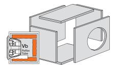
**Damping material:** FONOFORM on all the inside walls except for the speaker's.
